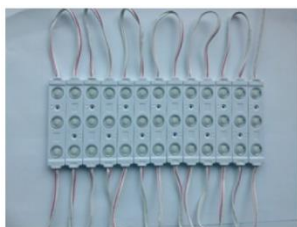
20 LED modules in a String
